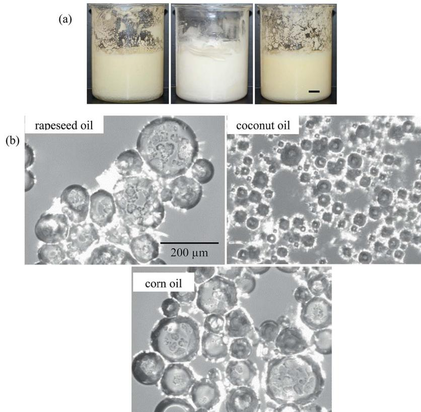
**Fig. 11** (a) Appearance of air-in-oil foams after whipping 5 wt% MA in oil at 22 °C for rapeseed oil (left), coconut oil (middle) and corn oil (right), scale bar = 1 cm and (b) corresponding optical micrographs, scale bar same in all cases.
