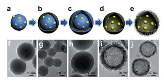
Fig. 2 Schematic illustration and TEM images of the formation process of PTM-HSs. (a) and (f) Pt loaded onto  $SiO_2$  nanospheres to form  $SiO_2$ -Pt. (b) and (g)  $TiO_2$  layers were coated on  $SiO_2$ -Pt to form  $SiO_2$ -Pt@ $TiO_2$ . (c) and (h)  $SiO_2$  protective layers were coated on  $SiO_2$ -Pt@ $TiO_2$  to form  $SiO_2$ -Pt@ $TiO_2$ @ $SiO_2$ . (d) and (i) PT-HSs. (e) and (j) PTM-HSs. The outermost spine-like layer in image (j) is the MnO<sub>x</sub> layer.
