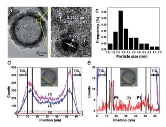
Fig. 3 The confirmation of PT-HS structures. (a) TEM image of a PT-HS. (b) HRTEM image of the area near the inner surface of the  ${\rm TiO_2}$  shell. (c) The distribution of the particle size. (d) EDS line scan of a PT-HS. The part in the dotted pane is magnified in image (e). (e) The magnified patterns of the EDS line scan. Inset in image (d) and (e): the path of the EDS line scan. Curves (1), (2) and (3) in image (d) and (e) refer to the signals of Ti, O and Pt, respectively.
