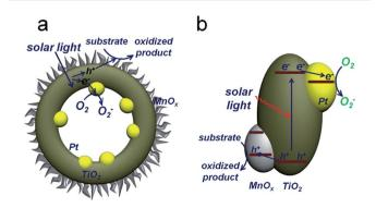
Fig. 1 Proposed mechanism for photocatalytic oxidation by PTM-HSs. Pt and  $MnO_x$  are spatially separated by  $TiO_2$ . (a) The reaction process. (b) Band structure of the catalyst.
