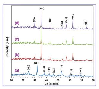
Fig. 1 XRD patterns of the as-synthesized  $CoCO_3/FeCO_3$  nanocomposite (a), and  $CoFe_2O_4$  products;  $S46\_400$  (b),  $S46\_500$  (c), and  $S46\_600$  (d).
