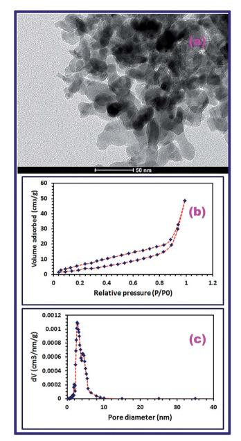
Fig. 8 TEM image of the  $CoFe_2O_4$  product (a),  $N_2$ -adsorption-desorption isotherm (BET) (b), and BJH pore size distribution (c).
