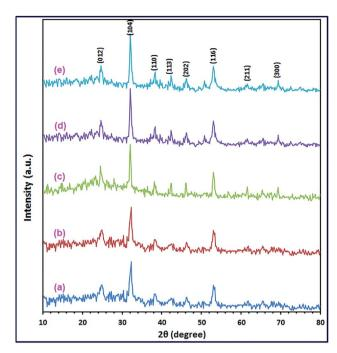
Fig. 3 XRD patterns of the as-synthesized  $CoCO_3/FeCO_3$  composites under hydrothermal reactions:  $Co^{2+}$ :  $Fe^{2+}$ : ascorbic acid:  $CO_3^{2-}$  molar ratio of 0.4:0.6:1:3, respectively, at 140 °C, for varying reaction times of 1.5 (a), 3 (b), 6 (c), 12 (d), and 24 h (e).
