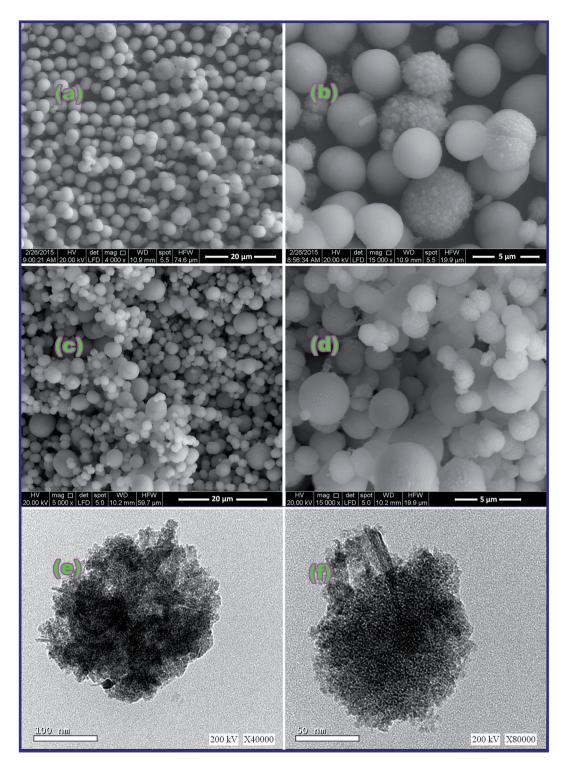
Fig. 4 FE-SEM images of the as-synthesized CoCO<sub>3</sub>/FeCO<sub>3</sub> nanocomposite (a and b) and CoFe<sub>2</sub>O<sub>4</sub> product (S46\_600 (c and d)); low and high magnification TEM images of CoCO<sub>3</sub>/FeCO<sub>3</sub> nanocomposite (e and f), respectively. where (a and c) are low magnification FE-SEM images, while (b and d) are high magnification FE-SEM images.
