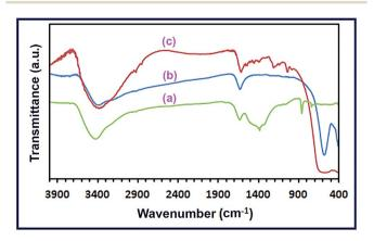
Fig. 5 FT-IR spectra of the as-prepared  $CoCO_3/FeCO_3$  nanocomposite (a), spinel  $CoFe_2O_4$  (b), and RR195-loaded  $CoFe_2O_4$  (c).
