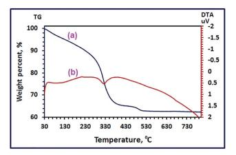
Fig. 6  $\,$  TG (a), and DTA (b) analyses of the as-prepared CoCO $_3$ /FeCO $_3$  nanocomposite under nitrogen gas.
