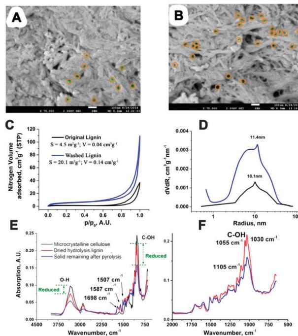
Fig. 4 (A) SEM of original CSHL x75000 with yellow encircled mesopores (B) SEM of washed CSHL x75000 with indicated mesopores (C) N<sub>2</sub> adsorption isotherms of washed/original CSHL. (D) Pore distribution derived from N<sub>2</sub> adsorption data for washed/original CSHL. (E and F) FT-IR of original CSHL (dried), the solid remaining after MW heating of CSHL and subsequent extraction of LGE (dried solid) and microcrystalline cellulose.
