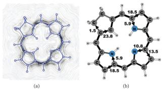
Fig. 5 (a) A streamline plot of the current density 1 bohr above the carbachlorin **19** molecule that sustains a net ring-current strength of 24.6 nA  $T^{-1}$  around the porphyrinoid macroring. (b) The calculated net current strengths (in nA  $T^{-1}$ ) passing selected bonds are given for carbachlorin **19**.
