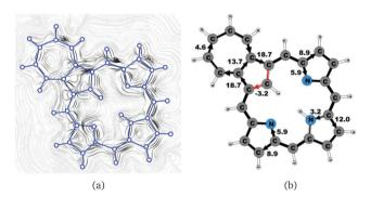
Fig. 13 (a) A streamline plot of the current density 1 bohr above the azuliporphyrin 3 molecule that sustains a net ring-current strength of  $15.1 \, \text{nA} \, \text{T}^{-1}$  around the porphyrinoid macroring. (b) The calculated net current strengths (in nA T<sup>-1</sup>) passing selected bonds are given for azuliporphyrin 3.
