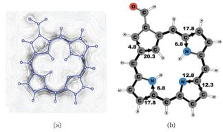
**Fig. 4** (a) A streamline plot of the current density 1 bohr above the carbaporphyrin **14** molecule that sustains a net ring-current strength of 24.6 nA  $T^{-1}$  around the porphyrinoid macroring. (b) The calculated net current strengths (in nA  $T^{-1}$ ) passing selected bonds are given for carbaporphyrin **14**.
