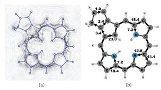
Fig. 10 (a) A streamline plot of the current density 1 bohr above the carbaporphyrin 9 molecule that sustains a net ring-current strength of 25.9 nA  $\mathsf{T}^{-1}$  around the porphyrinoid macroring. (b) The calculated net current strengths (in nA T<sup>-1</sup>) passing selected bonds are given for carbaporphyrin 9.
