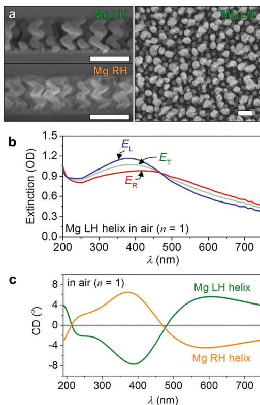
**Fig. 2** Mg nanohelices. (a) SEM images of Mg LH (left-top panel) and RH (left-bottom panel) nanohelices. The right panel shows the top view of the array of the Mg LH nanohelices (scale bar: 200 nm). (b) Extinction spectra of the Mg LH nanohelices in air in response to the unpolarised light ( $E_T$ , green) and the circularly polarised light (LCP:  $E_L$ , blue and RCP:  $E_R$ , red). (c) CD spectra of the 178 nm thick film containing LH (green) and RH (orange) Mg nanohelices in air.
