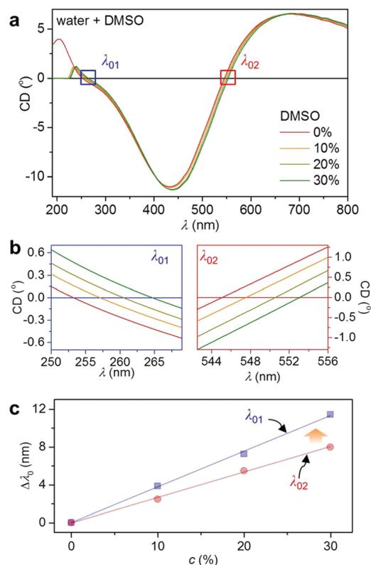
**Fig. 3** Molecular LSPR sensing. (a) CD spectra of Mg LH nanohelices in media with four different refractive indices (red: 0%, orange: 10%, yellow: 20%, and green: 30% DMSO–water mixtures) over the full spectral range and (b) detailed plots of the resonance shifts at  $\lambda_{01}$  (left panel) and  $\lambda_{02}$  (right panel). (c) Wavelength shift, relative to water, of the two spectral features as a function of the DMSO–water concentration.
