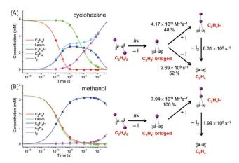
Fig. 7 Time-dependent concentration changes of chemical species (left) and schematic of the reaction mechanism (right) of the photodissociation reaction of  $C_2H_4I_2$  in (A) cyclohexane and (B) methanol.  $C_2H_4I$  radical (red),  $C_2H_4I-I$  isomer (green),  $C_2H_4$  (blue),  $I_2$  (cyan), and I atom (magenta). The points in the plot of concentration changes indicate the time delay points where the scattering data were measured.
