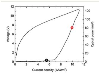
Fig. 3 Voltage vs. current density curve of the riQCL representing the emitted optical output power operated at 293 K (room temperature) driving the riQCL either at 5.5 kA cm<sup>-2</sup> (o: emission wavelength @ 1144 cm<sup>-1</sup>) or at 10 kA cm<sup>-2</sup> (o: emission wavelength @ 1144 cm<sup>-1</sup> and 1170 cm<sup>-1</sup>).
