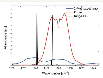
**Fig. 4** Laser emission lines (black) overlaid with the IR spectrum of furan (red), and 2-methoxyethanol (blue). The emission spectrum of the riQCL was obtained by coupling the emitted laser radiation into a Fourier transform infrared (FT-IR) spectrometer.
