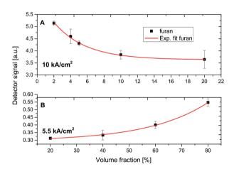
Fig. 6 riQCL-iHWG sensor system response to furan (in 2-methoxyethanol) obtained *via* selective emission line damping at an applied voltage of 10 kA cm<sup>-2</sup> (A), and of 5.5 kA cm<sup>-2</sup> (B). An exponential fit was applied to the response function resulting in a calibration model with a coefficient of determination ( $R^2$ ) >0.99 for both curves.
