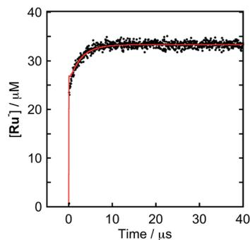
Fig. 8 Formation of Ru<sup>-</sup>: (a) DMF–TEOA (5 : 1 v/v) solution containing Ru (0.3 mM) and BI(OH)H (0.1 M) was irradiated at λ<sub>ex</sub> = 532 nm with a Nd:YAG pulse laser under degassed conditions at room temperature. The red line shows the fitting results (ESI†).
