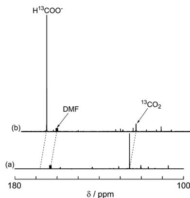
Fig. 3  $^{13}\text{C}\{^1\text{H}\}$  NMR spectra of the reaction solution before (a) and after (b) 13.5 h of irradiation:  $\text{DMF-}d_7\text{-TEOA}$  (4 : 1 v/v) solution containing  $\text{BI(OH)H}$  (0.1 M),  $\text{Ru}_2\text{-Ru(CO)}$  (0.5 mM), and  $^{13}\text{CO}_2$  (569 mmHg) was irradiated at  $>420 \text{ nm}$  using a xenon lamp.
