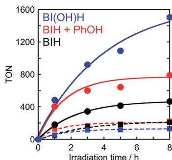
Fig. 10 Photocatalytic formation of formic acid (●) and CO (■) using BI(OH)H (0.1 M, blue), BIH and phenol (0.1 M each, red) or BIH (0.1 M, black): a  $\text{CO}_2$  saturated DMF-TEOA (4 : 1 v/v, 2 mL) solution containing  $\text{Ru}_2\text{-Ru(CO)}$  (0.025 mM), a sacrificial electron donor (0.1 M) and a proton source (0.1 M) was irradiated by  $\lambda_{\text{ex}} > 500$  nm light (LIC2).
