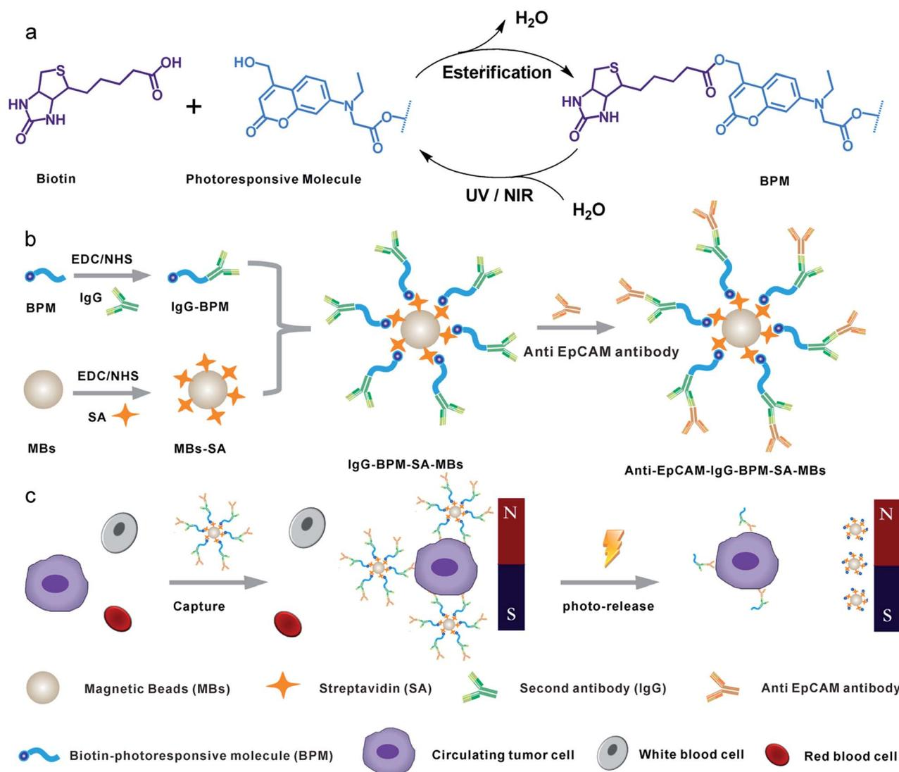
**Scheme 1** Schematic diagram showing the photoresponsive immunomagnetic system for capture and release of CTCs. (a) Synthesis and photo-induced cleavage of biotin-photoresponsive molecule (BPM); (b) construction of photoresponsive immunomagnetic beads; (c) capture and photo-induced release of CTCs.
