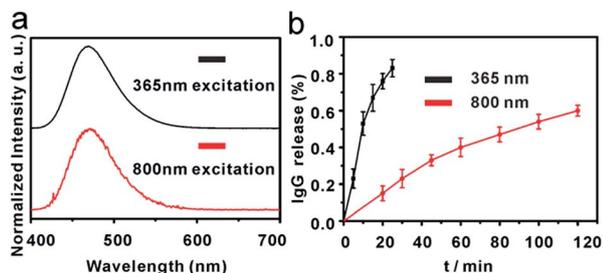
Fig. 1 (a) Emission spectra of compound 7 (upper: single photon excitation at  $365 \text{ nm}$ , lower: two photon excitation at  $800 \text{ nm}$ ); (b) time course of photolysis controlled IgG release from IgG-BPM-SA-MBs (left:  $365 \text{ nm}$ ,  $10 \text{ mW cm}^{-2}$ ; right:  $800 \text{ nm}$ ,  $10 \text{ mW cm}^{-2}$ ) (error bars represent standard deviations,  $n = 3$ ).
