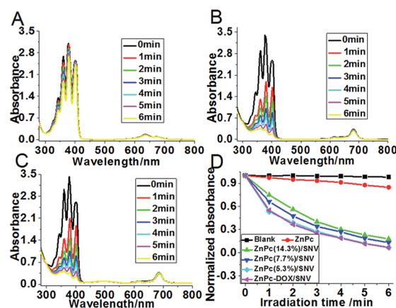
**Fig. 2** Decay curves of the ADPA absorbance in the presence of (A) ZnPc, (B) ZnPc(5.3%)/SNV and (C) ZnPc-DOX/SNV as a function of irradiation time (at 650 nm). (D) The normalized decay curves of the ADPA absorbance at 378 nm as a function of irradiation time, in the presence of pristine ZnPc, ZnPc( $x\%$ )/SNV, ZnPc-DOX/SNV as well as the blank measurement.
