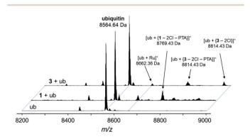
Fig. 5 Deconvoluted nESI-Q-TOF mass spectra of ubiquitin (8564.64 Da) and after incubation with  $\bf 1$  or  $\bf 3$  for 48 h. The mixture was incubated at a  $\bf 2:1$  metal-to-protein ratio in water.
