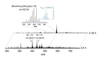
Fig. 6 ESI-IT mass spectra of  $\mathbf{1}$  in DMSO. The solution was diluted with water—methanol (1:1) prior to injection into the mass spectrometer.
