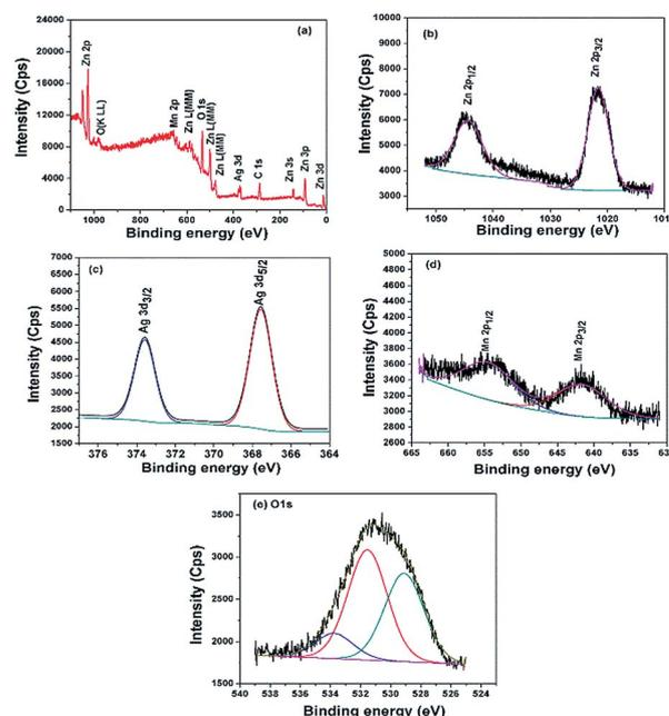
Fig. 3 XPS spectra of ternary ZnO/Ag/Mn<sub>2</sub>O<sub>3</sub> nanocomposite (a) survey, (b) zinc, (c) silver, (d) manganese and (e) oxygen.
