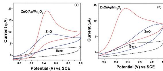
Fig. 6 The CV results of bare GCE and pure ZnO nanorods as well as ternary ZnO/Ag/Mn<sub>2</sub>O<sub>3</sub> nanocomposite modified GCE in presence of 3 mM (a) UA and (b) AA.
