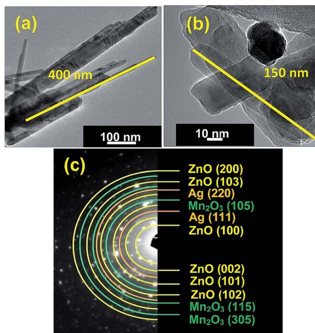
Fig. 2 TEM images of (a) pure ZnO, (b) ZnO/Ag/Mn<sub>2</sub>O<sub>3</sub> and (c) SAED pattern of ternary ZnO/Ag/Mn<sub>2</sub>O<sub>3</sub> nanocomposite.
