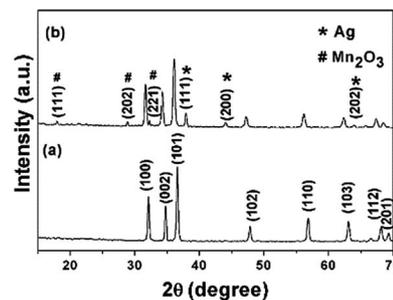
Fig. 1 XRD patterns of the synthesized (a) pure ZnO and (b) ternary ZnO/Ag/Mn<sub>2</sub>O<sub>3</sub> nanocomposite.
