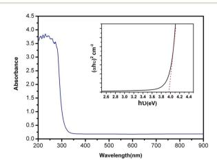
Fig. 1 UV-vis absorbance spectrum of the prepared ZnS:Cu-NP-AC (inset: plot of  $(\alpha h v)^2$  vs. (h v) for the prepared ZnS:Cu-NP-AC).
