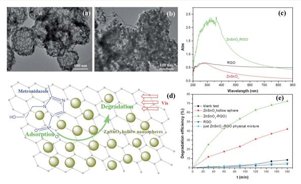
Fig. 3 The HRTEM images of the prepared  $ZnSnO_3$  hollow nanosphere (a) and  $ZnSnO_3/RGO$  nanocomposite (b). (c) The UV-Vis absorption spectra of the RGO, pure  $ZnSnO_3$  hollow nanosphere and  $ZnSnO_3/RGO$  nanocomposite. The speculated illustration (d) and degradation efficiencies (e) of the metronidazole wastewater by  $ZnSnO_3$  hollow nanosphere and  $ZnSnO_3/RGO$  nanocomposite photocatalysts under visible light irradiation. Reproduced with permission from ref. 33.
