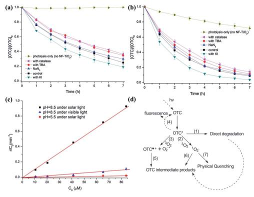
Fig. 5 Influence of TBA (10 mM), NaN $_3$  (5 mM), KI (10 mM) and catalase (6 unit per L) on the photocatalytic degradation of OTC by NF-TiO $_2$  under visible light at pH 5.5 (a) and 8.5 (b) (OTC 5 mg L $^{-1}$ ). (c) The initial rate of OTC photolytic degradation per unit of concentration at various initial concentrations at pH 5.5 and 8.5 under visible and solar light. (d) The proposed pathway of OTC photolytic degradation. Reproduced with permission from ref. 146.
