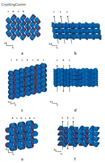
Fig. 3 Schematic representations of the packing arrangements of forms IP, IIP and IIIP with individual molecules shown as cones. Consecutive layers of forms IP, IIP and IIIP are laterally displaced as shown in (a), (c) and (e), respectively. Consecutive columns in  $I_P$  are oriented parallel to one another (b) while in forms II<sub>P</sub> (d) and III<sub>P</sub> (f) the columns are anti-parallel.
