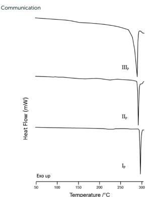
Fig. 5 DSC traces of forms  $I_P$  (bottom),  $II_P$  (middle) and  $III_P$  (top) heated at 10 K min<sup>-1</sup> in the range 25 to 315 °C.
