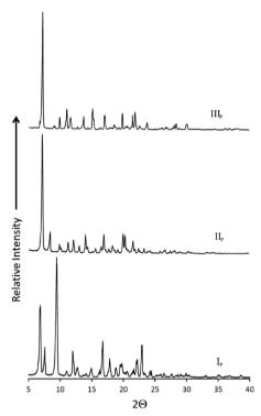
Fig. 6 Experimental powder X-ray diffraction patterns of forms  $I_P$  (bottom),  $II_P$  (middle) and  $III_P$  (top).
