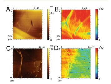
Fig. 6 AFM and EFM images. Topography of (A) A $\beta$  (16–23) and (C) F-A $\beta$ (16-23); electrostatic force map of (B) A $\beta$  (16-23) and (D) F-A $\beta$  (16-23). Peptides were 0.5 mg ml<sup>-1</sup> solutions in 10 mM phosphate buffer at pH 7.4 diluted 100-fold in ultrapure water and cast on Au-coated Si wafer.
