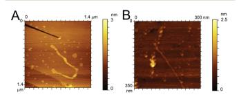
Fig. 4 AFM images of (A)  $A\beta$  (16–23) and (B) F- $A\beta$  (16–23), 0.5 mg ml<sup>-1</sup> in 10 mM phosphate buffer at pH 7.4 diluted 100-fold in ultrapure water cast and imaged on HOPG.
