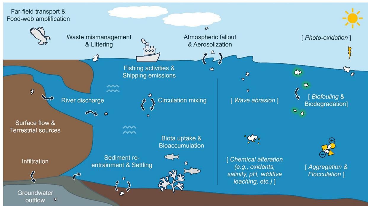
Fig. 1 Schematic overview of major transport (left) and transformation (right) pathways of plastic particles in aquatic systems.
