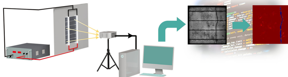
Fig. 1 PVEL image acquisition and machine learning-based defect segmentation.
