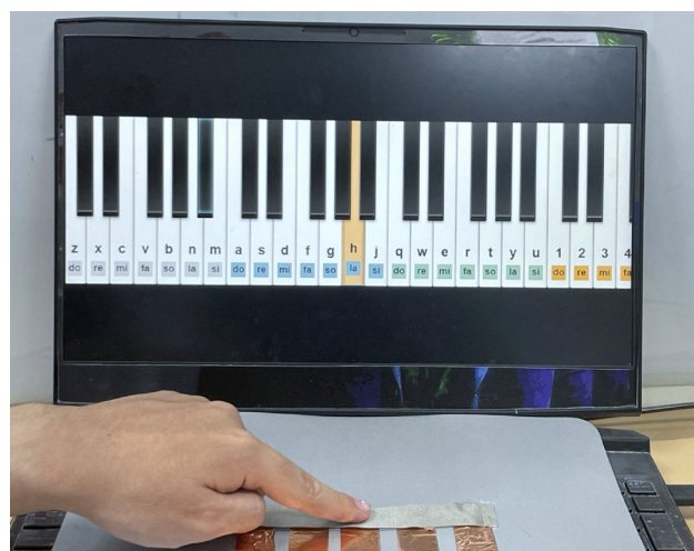
Fig. 8 Analysis of sensing performance using the piano of woven fabric electrode.
