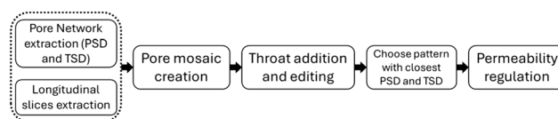
Fig. 1 Proposed steps for rock pattern design method.
