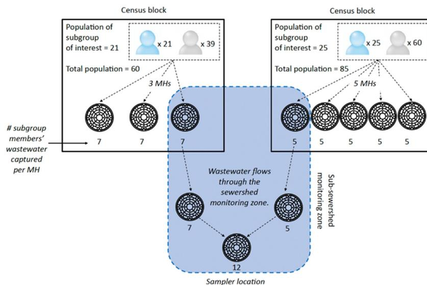
Fig. 3 Simplified illustration of the probabilistic assignment method adopted from Safford *et al.* (2022),<sup>17</sup> demonstrating how demographic data is distributed from a census block to a sub-sewershed zone.
