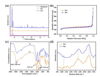
Fig. 3 (a) XRD curves of W1, W2, and standard UiO-66-NH<sub>2</sub>. (b) Nitrogen adsorption desorption curves for W1 and W2 at 77 K. Infrared (c) and Raman (d) spectra of W1 and W2
