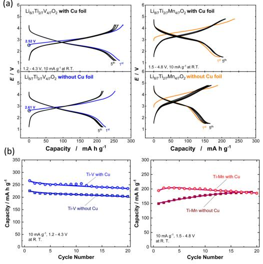
Fig. 3 (a) Galvanostatic charge/discharge curves and (b) discharge capacity retention for 20 cycles of  $Li_{8/7-x}Ti_{2/7}V_{4/7}O_2$  and  $Li_{8/7-x}Ti_{2/7}Mn_{4/7}O_2$  synthesized with or without Cu foil at a rate of 10 mA  $g^{-1}$ .
