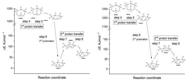
Energy diagrams of first and second proton transfer (steps 4-8) of Ni(PNP-C2-Me) 5a (left) and Ni(PNP-C2-H) 5b (right), calculated as DFT-PCM.
