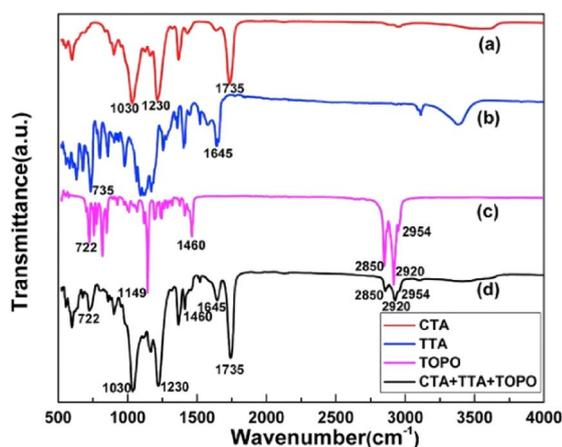
Fig. 8 FT-IR spectra of the (a) CTA blank membrane, (b) TTA, (c) TOPO, and (d) PIM respectively. Cai *et al.* (2019).<sup>68</sup> Copyright 2019 Elsevier.
