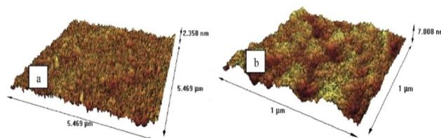
Fig. 5 AFM images of (a) pure PVC film and (b) PIM. Reused with permission from Kazemi *et al.* (2021).<sup>46</sup> Copyright 2021 Elsevier.
