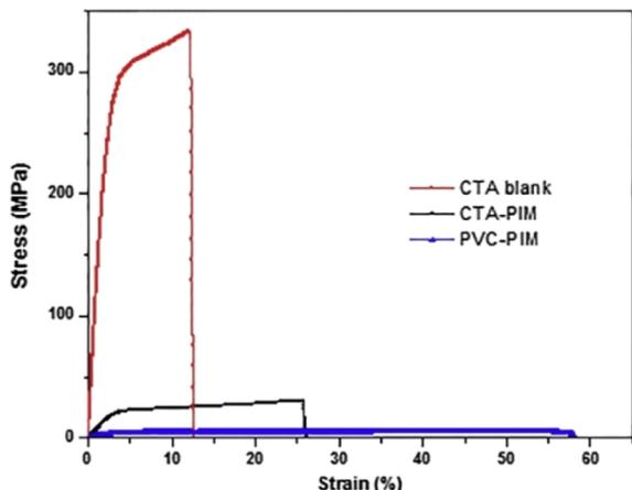
Fig. 6 Stress strain-curve of blank CTA, CTA based PIM, and PVC based PIM. Reused with permission from Nasser *et al.* (2016).<sup>102</sup> Copyright 2016 Elsevier.
