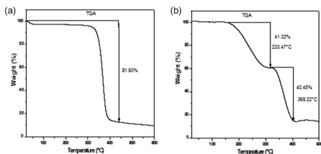
Fig. 7 Thermograms of: (a) CTA and (b) PIM. Nasser *et al.* (2016).<sup>102</sup> Copyright 2016 Elsevier.
