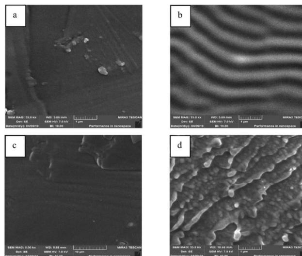
Fig. 4 SEM images of the surface and the cross section of the PVC film (a and c), and the 50% D2EHPA PIM (b and d). Reprinted with permission from Kazemi *et al.* (2021).<sup>46</sup> Copyright 2021 Elsevier.
