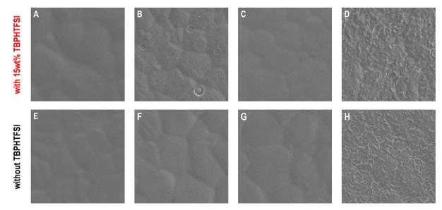
Fig. 4 Top-view scanning electron microscopy images of the organic semiconductor—TBPHTFSI composite layers deposited on the surface of FAPbI $_3$  perovskite polycrystalline thin films and the corresponding pristine organic semiconductor layers: (A and E) spiro-OMeTAD, (B and F) p-DTPF4, (C and G) p-DTPF4-EBEH, (D and H) p-EBEH. Image size: 5  $\mu$ m  $\times$  5  $\mu$ m. Encapsulation materials and gold electrodes were removed before imaging.
