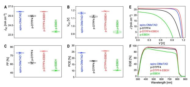
Fig. 3 (A–D) Statistical analysis of photovoltaic parameters of PSCs fabricated with varying hole transport layers under simulated AM1.5G irradiation at 100 mW cm<sup>-2</sup>: (A) short-circuit photocurrent density ( $J_{SC}$ ); (B) open-circuit voltage ( $V_{OC}$ ); (C) fill factor (FF); (D) power conversion efficiency (PCE). (E) Representative photocurrent density-voltage (J-V) curves. (F) External quantum efficiency (EQE) spectra.
