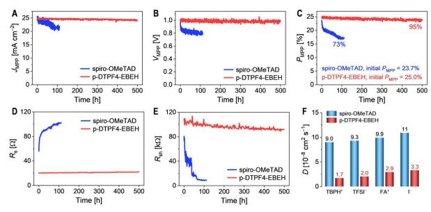
Fig. 7 (A–C) Photovoltaic parameters obtained from maximum power point (MPP) tracking under simulated AM1.5G irradiation at 100 mW cm<sup>-2</sup>: (A) photocurrent density ( $J_{MPP}$ ); (B) photovoltage ( $V_{MPP}$ ); (C) power conversion efficiency ( $P_{MPP}$ ). (D and E) Evolution of series resistance ( $R_s$ ) and shunt resistance ( $R_{sh}$ ) over time during MPP tracking. (F) Diffusivities of ions within the hole transport layer at 45 °C.
