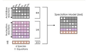
Fig. 1 Schematic example of the equations arising from a simple reaction network for one monomer M1 giving a dimer M2, and their protonated forms, so a total of 6 species, 4 acid/base reactions in grey, 6 nucleation reactions in purple, plus the mass balance equation in orange.
