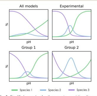
Fig. 3 Simplified example of a three-species speciation diagram, showing an average diagram for the whole set of SMs (top left), the experimental reference (top right), and two clusters obtained through K-means clustering and filtering (bottom).
