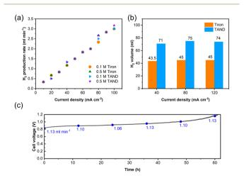
**Fig. 3** Cell characterization at different current densities and concentrations. (a) Hydrogen production rate during stepwise-LSV at concentrations 0.1 M/0.5 M. (b) Collected hydrogen volume in higher current densities using 10 ml of 0.1 M Tiron/TAND in 1 M  $\rm H_2SO_4$ . (c) Performance of long-term electrolysis using 2 liters of 0.1 M TAND electrolyzed at 40 mA cm $^{-2}$ . Gas production rates (ml min $^{-1}$ ) are depicted every 12 hours.
