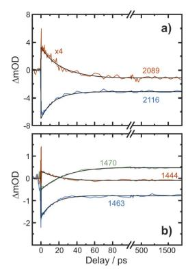
Fig. 6 Pump-probe kinetic traces recorded in (a) the azide antisymmetric-stretch region and (b) in the CN/CH-region. The black curves represent fits of the transients to single-exponential kinetics.
