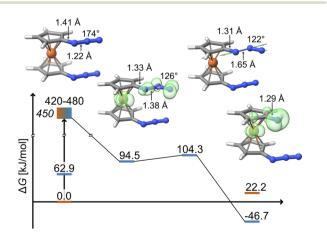
Fig. 4 Gibbs free energy profile in kJ mol<sup>-1</sup> for the photolytic N<sub>2</sub> dissociation pathway proposed by DFT (D4-PBE0/def2-TZVP). The experimental irradiation energy is given in italics. Loewdin spin populations for the intermediate, Fe: 1.1,  $(N_{\alpha}, N_{\beta}, N_{\gamma})$ : (0.2, 0.2, 0.6), and product, Fe: 0.6, N: 1.1.
