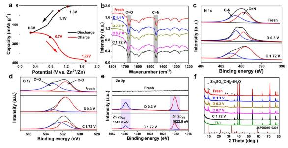
Fig. 5 (a) Charge and discharge profiles of TA-PTO-COF at a current density of  $0.1 \, \text{A g}^{-1}$ . (b) Ex situ FT-IR spectra of the TA-PTO-COF cathode at different potentials. Ex situ XPS analysis of (c) N 1s, (d) O 1s, and (e) Zn 2p. (f) Ex situ XRD patterns of the TA-PTO-COF cathode at different potentials.
