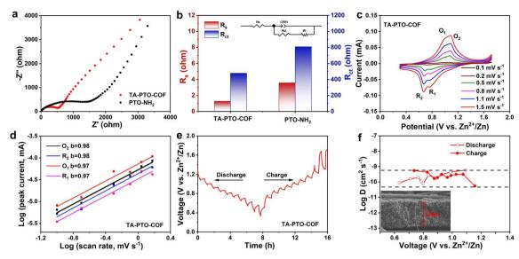
Fig. 4 (a) EIS plots of PTO-NH<sub>2</sub> and TA-PTO-COF. (b) Impedance fitting diagram of PTO-NH<sub>2</sub> and TA-PTO-COF. (c) CV curves of the TA-PTO-COF cathode at various sweep rates. (d) *b* values of TA-PTO-COF. (e) GITT curves of the TA-PTO-COF electrode (first charge/discharge state). (f) Corresponding quantified  $D_{Zn}^{2+}$  at different potential stages and the SEM image of a TA-PTO-COF electrode section.
