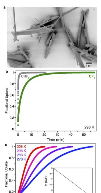
Fig. 6 (a) SEM image of sieved Zn(fba) showing a wide dispersity of crystallite sizes. (b) Transient adsorption data for CF<sub>4</sub> (green) or CHF<sub>3</sub> (grey) adsorption in Zn(fba) following a 1.00 mmol  $g^{-1}$  dose at 298 K. (c) Variable temperature CF<sub>4</sub> transient adsorption data from which values of  $D/l^2$  were calculated. The inset shows the Arrhenius plot from which the activation energy of diffusion was determined.
