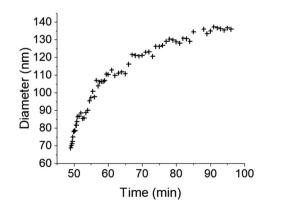
Fig. 5 Evolution of the IO@STMS NP final diameters measured on the in situ LPTEM images from ESI Video 2.†
