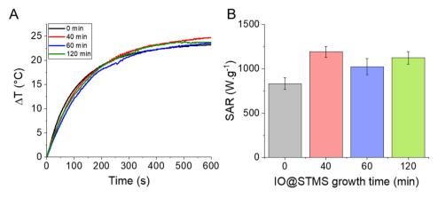
Fig. 11 (A) Temperature profiles as a function of time for the different IO@STMS-t NPs at 0.5 mgFe mL<sup>-1</sup> under NIR light irradiation. (B) Corresponding SAR values. These results were obtained with the IO@STMS-t obtained from series 2.
