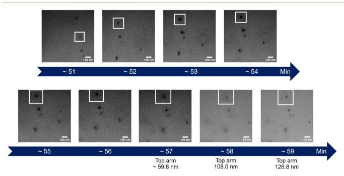
Fig. 3 Time-lapse images extracted from the in situ LPTEM video ESI Video 1.† The white box represents an interesting particle whose diameter is measured on the last images.
