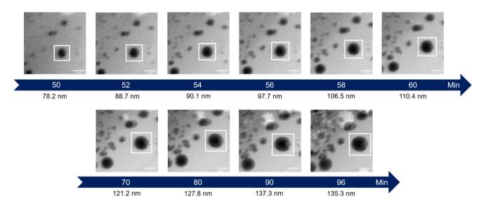
Fig. 4 Time-lapse images extracted from the in situ LPTEM video ESI Video 2.† The white box shows the particle whose diameter is indicated under the images.
