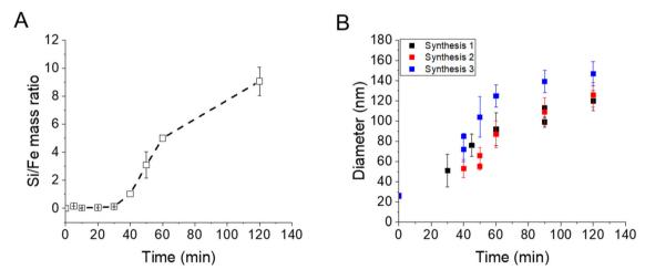
Fig. 2 (A) Kinetic tracking of STMS growth on IO NPs by Si/Fe mass ratio obtained by EDX. (B) Evolution of the IO@STMS NP final diameters measured by TEM on three different syntheses.
