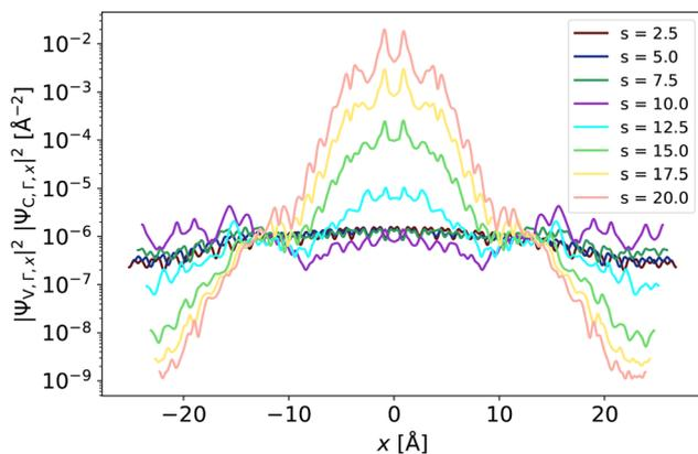
**Fig. 9** Product of the WFD at the frontier states, plotted on a logarithmic scale. Strong localization at higher values of strain leads to a very large overlap of the wave functions. The V and C indices denote valence and conduction bands, respectively.
