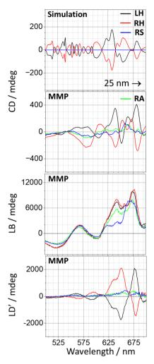
Fig. 10 A comparison between simulated CD and MMP measured CD, LB and LD' for a 210 nm sample. The MMP CD data has been smoothed to aid comparison
