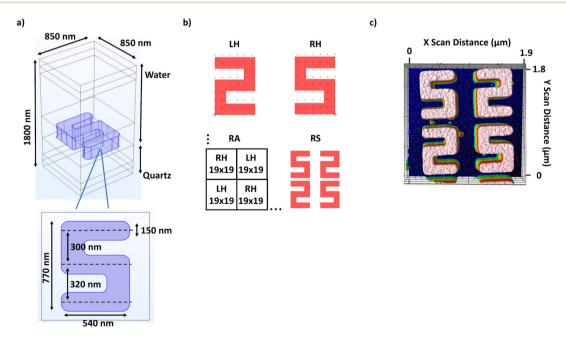
Fig. 1 (a) The unit cell containing an idealised RH geometry used to model the structures in numerical simulations, with labelled feature sizes. (b) Designs for the repeating units of each array are illustrated. (c) An AFM image of LH and RH structures as part of the RS array.
