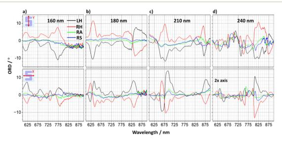
Fig. 8 Experimental ORD spectra obtained for y-(top) and x-polarised (bottom) LPL for 160-240 nm sample heights, (a)-(d). Note the increased scale of the 240 nm data.
