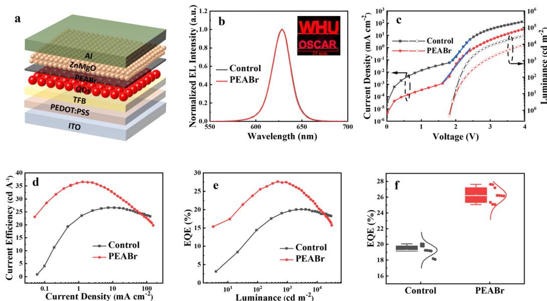
Fig. 2 (a) Schematic diagram of the PEABr-based device structure. (b) Normalized EL spectra. Inset: Photo of two operating PEABr-based QLEDs with different logos. (c)  $J$ – $V$ – $L$ , (d) CE, and (e) EQE curves of the device with and without PEABr. (f) Numerical distributions of the EQEs measured from 10 devices, respectively.
