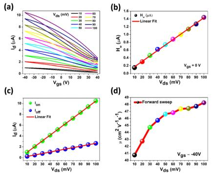
Fig. 3 (a) Transfer characteristics, (b) hysteresis width, (c) on and off current values at  $V_{\rm gs} = -40$  V and  $V_{\rm gs} = 40$  V, respectively, and (d) calculated mobility as a function of the drain voltage at  $V_{\rm qs} = -40$  V, RT and 2 mbar pressure. Line in (d) is guide to the eye.
