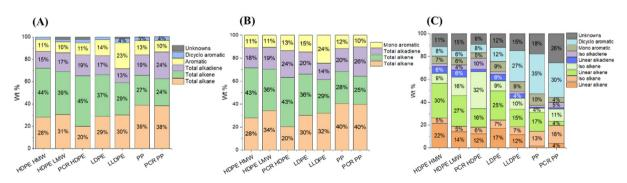
Fig. 4 The overall summary of oil weight percentage distributions of (A) whole oil, (B) light oil, and (C) heavy oil with branch analysis for all 7 plastic pyrolysis oils, quantified through  $GC \times GC$ -FID.
