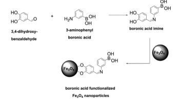
Fig. 15 Functionalization of  $Fe_3O_4$  nanoparticles with boronic acid moieties performed by Mohapatra *et al.* This figure has been reproduced from ref. 80 with permission from the Elsevier, copyright 2009.
