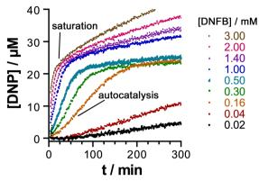
Fig. 6 Progress of the S<sub>N</sub>Ar reaction of DNFB (0.02–4.4 mM) with 0.01 M H as catalyst (pH 8.6, borate buffer) showing both autocatalysis at low substrate concentrations - note the characteristic sigmoidal shape of the reaction progress curve - and saturation of the cavity by product at high concentrations.
