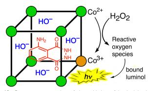
**Fig. 12** Cartoon representation of the oxidation of luminol by  $H_2O_2$  catalysed by the cage  $\mathbf{H^w}$  which (i) binds the guest, (ii) uses its  $Co(\shortparallel)/Co(\shortparallel)$  redox couple to activate the  $H_2O_2$  generating reactive oxygen species surrounding the cage surface, and (iii) tethers any hydroxide ions required for the reaction in place via the cage positive charge.
