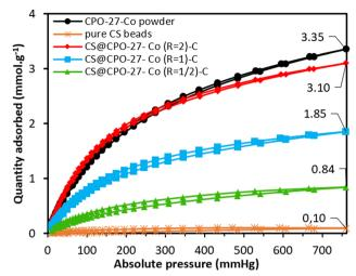
Fig. 3 CO<sub>2</sub> adsorption isotherms of the as-synthesized CPO-27-Co powder, pure CS beads, and CS@CPO-27-Co (R) beads measured at
