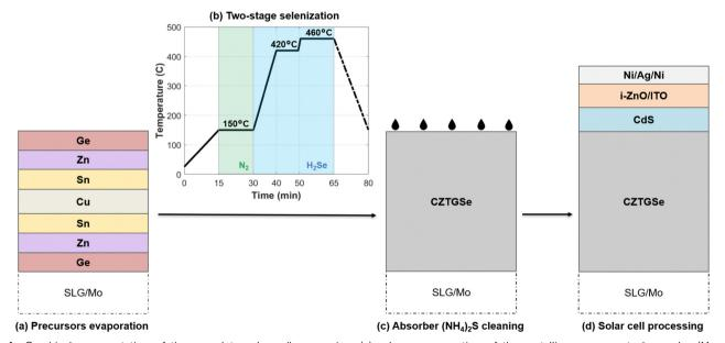
Fig. 1 Graphical representation of the complete solar cell processing: (a) e-beam evaporation of the metallic precursor stack on glass/Mo. (b) Temperature profile of the two-step  $H_2$ Se annealing with pre-annealing in  $N_2$ . (c)  $(NH_4)_2S$  cleaning treatment applied on the absorber's top surface. (d) Deposition of the CdS buffer, i-ZnO/ITO window layers, and Ag grid to complete the solar cell process
