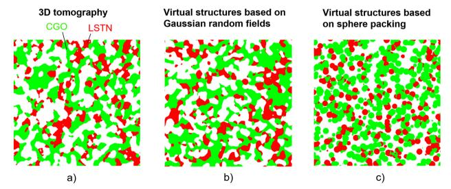
Fig. 2 Comparison of a real *versus* two virtual microstructures (illustrated with 2D orthoslices from 3D structures): (a) segmented tomography data representing a real LSTN-CGO structure with continuous phases, (b) virtual reconstruction of the LSTN-CGO microstructure based on a pluri-Gaussian method (PGM) providing a good match to the real microstructure and (c) virtual reconstruction with sphere packing (not well suited for SOFC electrodes).
