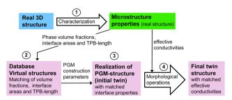
Fig. 10 Workflow for the construction of a digital microstructure twin for a corresponding real structure, e.g., from tomography. (1) Characterization of the real structure, (2) determination of the PGM parameters for matching microstructure properties, (3) generation of an initial PGM structure and (4) optimization of the relative conductivities with morphological
