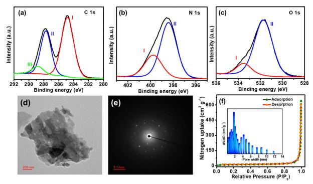
Fig. 1 Core level XPS spectra for (a) C 1s, (b) N 1s, and (c) O 1s of TP-COF. (d) TEM images and (e) corresponding SEAD image of TP-COF. (f)  $N_2$  adsorption-desorption analysis of TP-COF and the corresponding pore size distribution plot of TP-COF in the inset.
