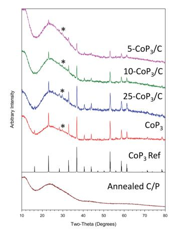
Fig. 2 Powder XRD results for x-CoP<sub>3</sub>/C (x = 5, 10, 25 mol%) products from two-step synthesis procedure of methanol precipitations of x-CoCl<sub>2</sub>/ C (x = 5,10, 25 mol%) followed by direct reactions of x-CoCl<sub>2</sub>/C with elemental red phosphorus at 500 °C. Reference (Ref) pattern for CoP<sub>3</sub> and XC-72 carbon black annealed at 500 °C with elemental red phosphorus are also shown. Trace CoP<sub>2</sub>O<sub>6</sub> impurity are identified with a (\*).
