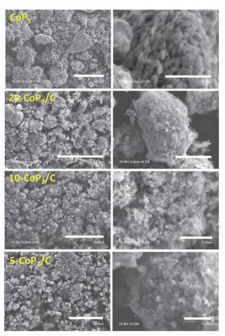
Fig. 4 Representative SEM images of CoP<sub>3</sub> and x-CoP<sub>3</sub>/C (x = 5, 10, 25 mol%) powders from reactions of x-CoCl<sub>2</sub>/C and red phosphorus at 500 °C. Scale bars are 50  $\mu$ m for all left images. Scale bar lengths for right images of CoP<sub>3</sub> and 10-CoP<sub>3</sub>/C are 5  $\mu$ m and 25-CoP<sub>3</sub>/C and 5-CoP<sub>3</sub>/C are 10  $\mu$ m.
