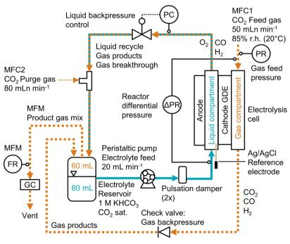
Fig. 1 Process flow diagram for CO2 electrolysis setup. The backpressure of the electrolyte stream was controlled (PC) before it was mixed with the purge gas and recirculated. The differential pressure,  $\Delta p$ , across the GDE was measured between the catholyte and gas compartment ( $\Delta$ PR). The Faradaic efficiency was determined by recording the product gas flow rate (FR) with a mass flow meter (MFM) and analyzing the gas composition by gas chromatography (GC).
