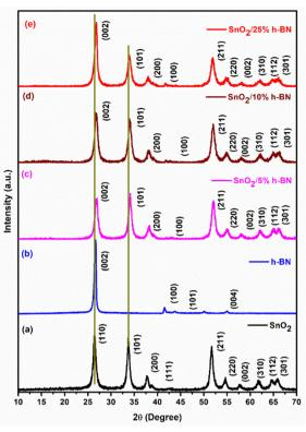
Fig. 1 XRD patterns of (a)  $SnO_2$ , (b) h-BN, (c)  $SnO_2/5\%$  h-BN, (d)  $SnO_2/5\%$ 10% h-BN and (e) SnO<sub>2</sub>/25% h-BN composites
