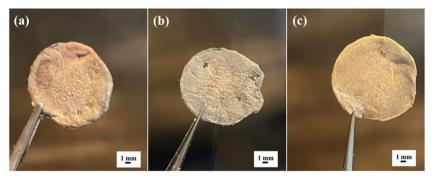
Fig. 5 Digital photograph of the lithium metal anodes after 350 charge/discharge cycles at 1C rate: (a) lithium anode with the  $SnO_2/5\%$  h-BN composite separator, (b) lithium anode with the  $SnO_2/25\%$  h-BN composite separator and (c) lithium anode with the  $SnO_2/25\%$  h-BN composite separator.
