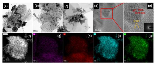
Fig. 3 (a-c) TEM images of SnO<sub>2</sub>/10% h-BN, (d) HRTEM image, and (e) SAED of SnO<sub>2</sub>/10% h-BN (bright field); (f) TEM image and the corresponding (g) boron, (h) nitrogen, (i) tin, and (j) oxygen EDX elemental mappings of a SnO<sub>2</sub>/10% h-BN particle.
