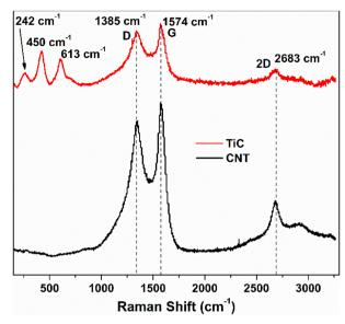
Fig. 3 Raman spectra collected from two samples at a laser excitation wavelength of 532 nm: (black) standard CNT/Fe/Al<sub>2</sub>O<sub>3</sub>/Cu sample where CNTs were grown by CVD and (red) the sample without the Fe catalyst resulting in no CNT growth but verifying the presence of the TiC interface.
