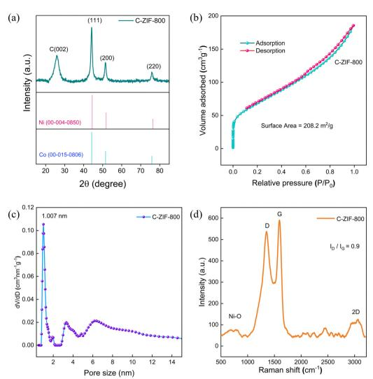
Fig. 1 (a) PXRD patterns of C-ZIF-800. (b)  $N_2$  sorption isotherm of C-ZIF-800. (c) BHJ pore size distributions of C-ZIF-800. (d) Raman scattering spectrum of C-ZIF-800.
