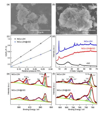
Fig. 1 Surface morphology and characterization of the prepared electrocatalyst. (a) SEM images of NiCo-LDH, (b) SEM image of NiCo-LDH@GO, (c) BET surface area of NiCo-LDH and NiCo-LDH@GO, (d) PXRD pattern for rGO, NiCo-LDH, and NiCo-LDH@GO. (e) Ni 2p XPS peak for NiCo-LDH and NiCo-LDH@GO, and (f) Co 2p XPS peak for NiCo-LDH and NiCo-LDH@GO
